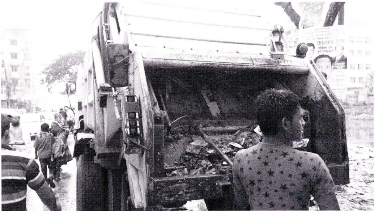
Figure 4.6: Transportation of SW by covered truck in Dhaka
