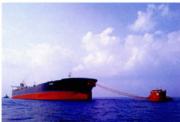
Figure 7: Installation of Single Point Mooring (SPM)
