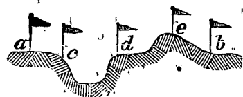
Fig. 139.—Ranging Long Line across Elevations and Depressions.
